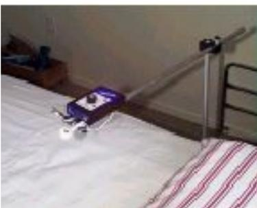
Although many commercial systems exist, sometimes switches need to be mounted in a way that requires a custom solution. The first example shows a switch mounting bracket for a client's bed at home; additional components allow the switch to be easily mounted on the client's wheelchair also. The second example is a simple gooseneck holder which has been adapted to hold a switch or a ventilator mouthpiece
