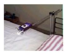
Although many commercial systems exist, sometimes switches need to be mounted in a way that requires a custom solution. The first example shows a switch mounting bracket for a client's bed at home; additional components allow the switch to be easily mounted on the client's wheelchair also. The second example is a simple gooseneck holder which has been adapted to hold a switch or a ventilator mouthpiece
