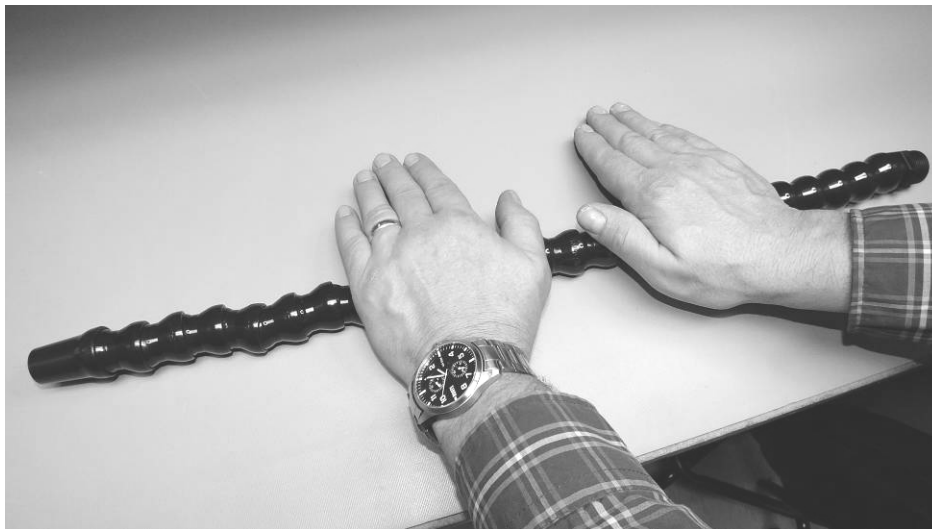
Figure 3. Straighten the arm by rolling on a flat surface.
