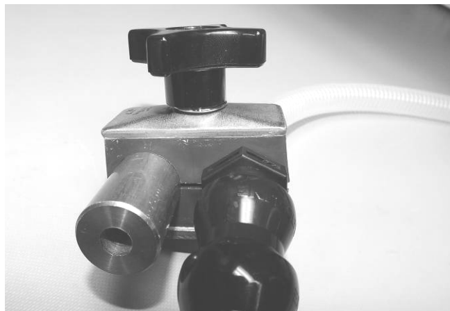
Figure 5. CANVent arm clamped to tubing.
