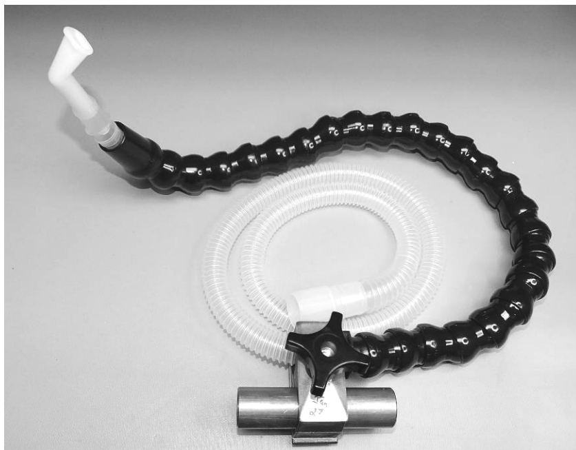
Figure 6. CANVent arm with mouthpiece installed.
